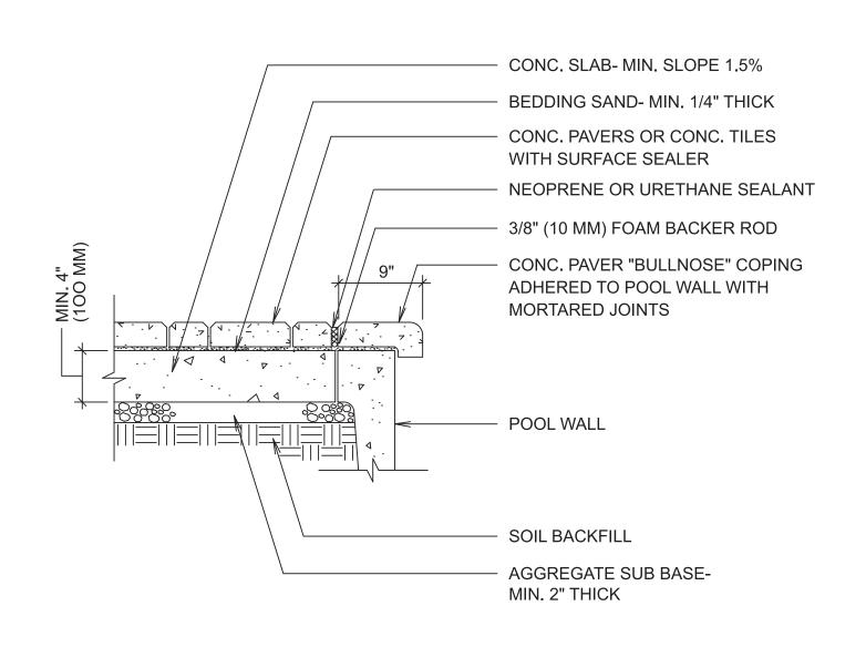
NOTE: COVER JOINTS WITH GEOTEXTILE AND FILL ALL CRACKS TO PREVENT LOSS OF BEDDING SAND
